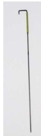
The Hanksraft switch machine shaft has a 1/16" hole in it, into which I insert a piece of brass rod. I bend one end of the rod into a loop, and solder the rod to the shaft.
