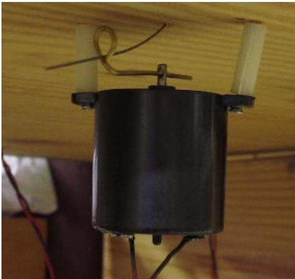
To install the motor, I run the control lever through the loop in the brass rod, and attach the motor to the bottom of the layout with #4 screws I run through the mounting "ears" in the motor and 1 1/4" nylon standoffs I print on my 3D printer. I connect the wires from the motor to a Digitrax DS44
