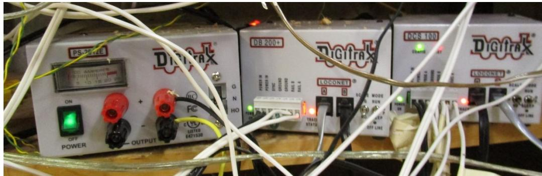
The booster in the middle is connected to a Digitrax PM42 to manage power to different sub-districts.
